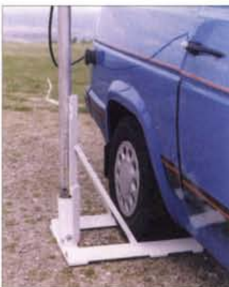
Fig. 5: The prototype 'TEX' version in use with the Reliant three wheel car. The mast is about to be 'locked' into the vertical position with the top clamp (note that prototype was painted, the production version will be 'hot dipped' galvanised (see text)).
