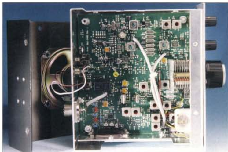
Fig. 11: An inside view of the MFJ-9402. The ladder filter can be seen at the top right (see text).
