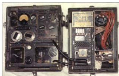
Fig. 7: The B2 in its metal box version, both boxes had close-fitting lids and were suitable for a parachute drop. (Photograph B. Warner).
