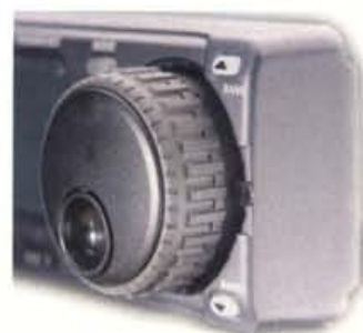
Fig. 3: The main tuning knob has a friction brake which increases the tension on the knob which Richard G0RSN says makes a big difference when you are operating from the car.
