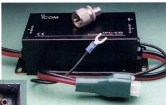
Fig. 7: The EMC filter box of the Icom IC-706 MkIIG and (inset) the inside view.
